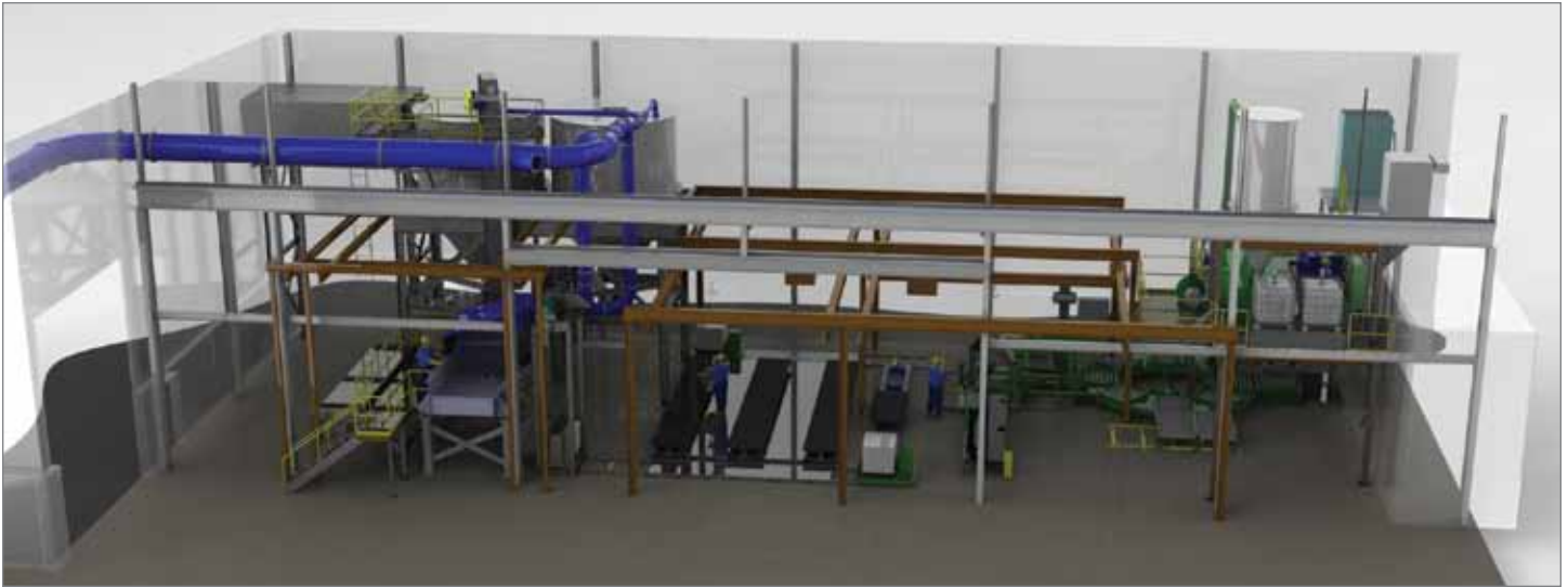
No Bake System Installation
